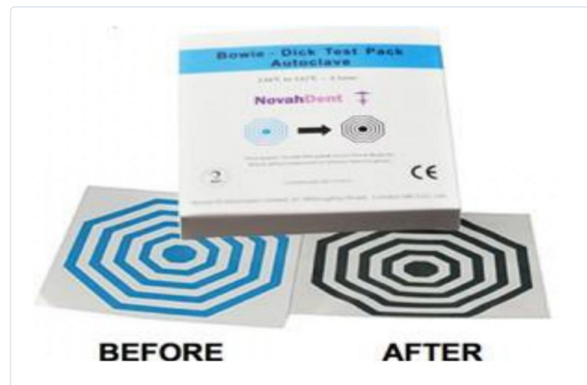
Fig. 3 — HELIX / Bowie-Dick chemical indicator: blue before the cycle, uniformly dark after adequate steam penetration.
